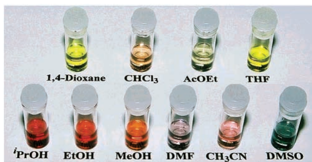
Figure 3. Solvatochromism between host 1 and various solvents. The concentration of host 1 was 1.0 \times 10^{-3} M in the presence of n -hexylamine ( 1.0 \times 10^{-1} M) at 25 °C.
