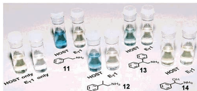
Figure 10. Color development by the hosts 1 and 2 with various amines. The concentration of hosts 1 and 2 were 1.0 \times 10^{-3} M and those of amines 11–14 were 1.0 \times 10^{-1} M in DMSO at 25 °C: 11 , phenethylamine; 12 , 1-amino-2-phenylpropane; 13 , 2,2-diphenylethylamine; 14 , 2-amino-1-phenylethanol.
