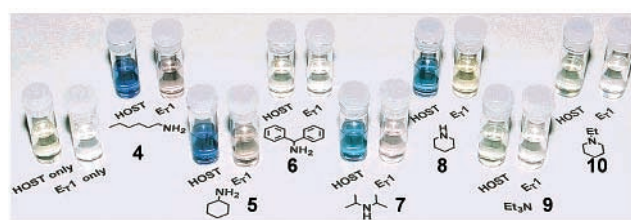
Figure 8. Color development by the hosts 1 and 2 with various amines. The concentration of hosts 1 and 2 were 1.0 \times 10^{-3} M and those of amines 4–10 were 1.0 \times 10^{-1} M in DMSO at 25 °C: 4 , n -hexylamine; 5 , cyclohexylamine; 6 , benzhydrylamine; 7 , diisopropylamine; 8 , piperidine; 9 , triethylamine; 10 , n -ethylpiperidine.
